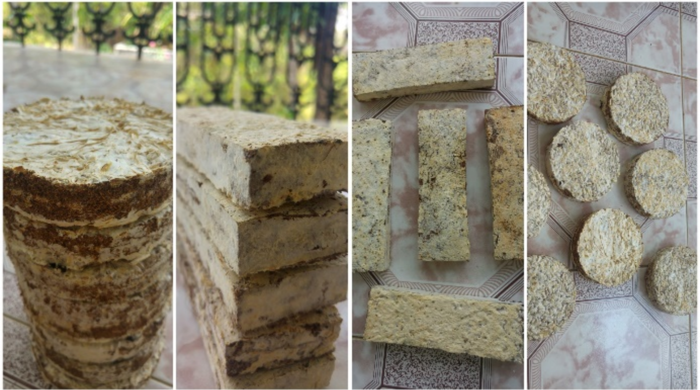
Figure 5: Top views and side views of the fabricated MBCs used for different tests.
